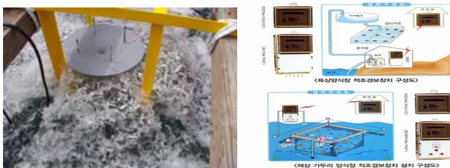
Fig. 4. Bottom water pumping in the cages, and red tide alarm system and schematic layout in the land-based fish tank (up) and fish cage(down) to alert aquaculture manager(NFRDI, 2002).
