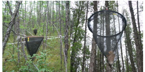
Litter traps for evaluating carbon dynamics in Siberian larch forest (L) and Canadian pine stand (R).
